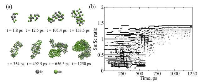
Fig. 3 (a) Snapshots of the heaviest  $Sn_xSe_y$  cluster during growth. (b) Stoichiometric ratios of the 10 heaviest  $Sn_xSe_y$  clusters in the system at each time interval
