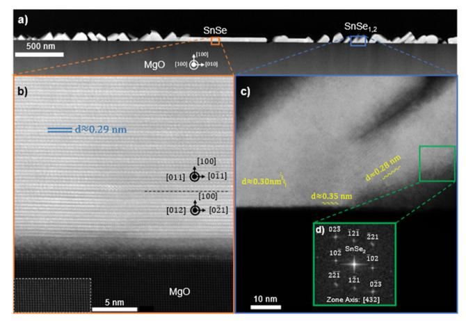
Fig. 6 HAADF STEM images of SnSe film on MgO at a 1:4 Sn: Se flux ratio at 270 °C for 6 hours at (a) the interface between MgO and SnSe highlighting both flat in-plane growths and angled out-of-plane structures; a magnified image of (b) a region with (200) out-of-plane orientation and (c) a region with a (210) out-of-plane orientation (a); (d) an SAED pattern of a region of SnSe<sub>2</sub>. The region in the dashed white box is a high contrast section of (a) to better illustrate the cubic MgO.
