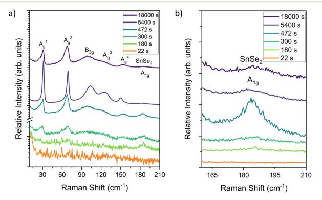
Fig. 5 Raman spectra of *Pnma* SnSe thin films taken for different deposition times across (a) the full range of vibrational modes and (b) focused on the region indicating the SnSe<sub>2</sub> A<sub>1q</sub> mode.
