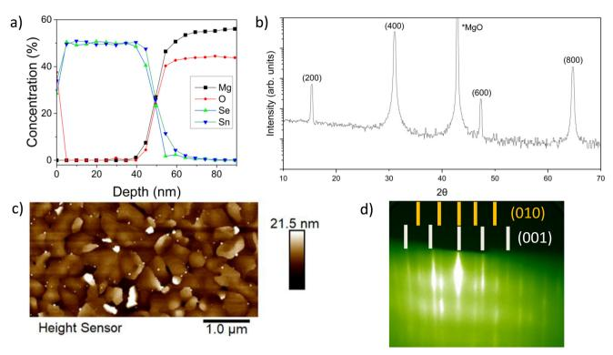
Fig. 2 (a) XPS depth profile of a SnSe thin film deposited on MgO with 1:4 Sn: Se flux ratio at 280 ± 5 °C for 83 minutes. (b) XRD of the film in 2a indicating (200) orientation out-of-plane, (c) AFM on the same film showing mixed orientation distribution in-plane, and (d) RHEED measurements of a SnSe film with multiple in-plane orientations taken post growth.
