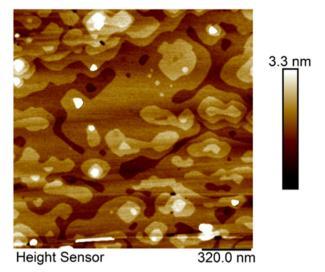
Fig. 7 SnSe thin film grown on MBE at 285 °C for 30 min. There are large lateral regions. The step height between islands is approximately 0.6 nm which matches the monolayer of SnSe.
