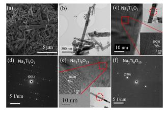
Fig. 3 (a) SEM image of the mixed phase rods, (b) low-resolution TEM image of the rods, (c) HRTEM image of a  $Na_2Ti_3O_7$  rod with inset low-resolution image and one to resolve lattice fringes, (d) corresponding SAED pattern, (e) HRTEM image of a  $Na_2Ti_6O_{13}$  rod with low-resolution inset image to resolve lattice fringes, (f) corresponding SAED pattern.
