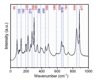
Fig. 2 Raman spectrum of NTO sample, the red arrows correspond to the  $Na_2Ti_3O_7$  phase and blue arrows  $Na_2Ti_6O_{13}$ .
