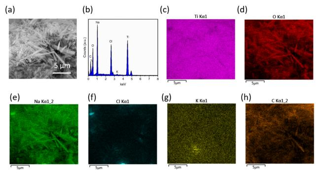
Fig. 4 (a) SEM image of the mixed phase rods, and ((b)) corresponding EDX spectrum. EDX elemental maps of (c) Ti, (d) O, (e) Na, (f) Cl, (g) K, and (h) C. According to the EDX mapping Na, Ti, and O are distributed uniformly and taking a major role in the synthesized product. However, Cl and K are also present in the sample as contaminant product that are coming from IL.
