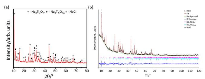
Fig. 1 (a) XRD pattern of as-prepared  $Na_2Ti_3O_7$  (represented with a star symbol). The secondary phase is indicated using a filled diamond ( $Na_2Ti_6O_{13}$ ) with the NaCl impurity represented by a filled circle symbol. (b) Rietveld refinement of the sample, (black symbols experimental pattern; red line calculated pattern; blue line difference curve, with a reduced  $\chi^2$  of 3.77.
