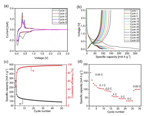
Fig. 5 Electrochemical performance of NTO electrodes (a) cyclic voltammogram curves in a voltage range of 0.0-3.0 V at a scanning rate of 0.08 mV s<sup>-1</sup>, (b) charge-discharge profiles in a voltage range of 0.01-2.5 V at current density of 10 mA g<sup>-1</sup>, (c) cycling performance of NTO electrode at current density of 10 mA g<sup>-1</sup> (d) rate capability of NTO electrode.
