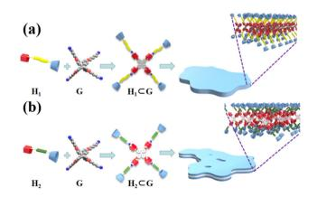
Fig. 10 Formation of host-quest complexes (a)  $H_1 \subset G$  and (b)  $H_2 \subset G$ , and self-assembly in CHCl<sub>3</sub>/DMSO solution, respectively.
