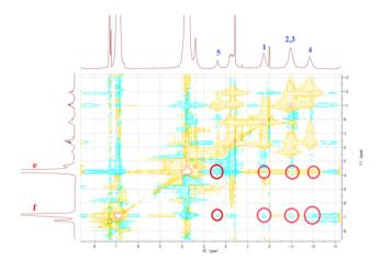
Fig. 7  $^{1}H^{-1}H$  NOESY NMR spectrum (500 MHz) of the complex of G with  $H_3$  at a 1:4 molar ratio in CDCl<sub>3</sub> at 25  $^{\circ}$ C.
