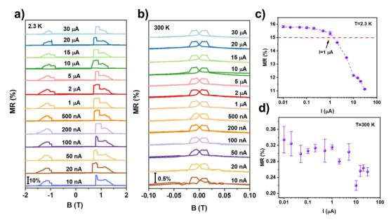
Fig. 4 Bias-current-dependence of the spin-valve effect in the Fe<sub>3</sub>GaTe<sub>2</sub>/MoS<sub>2</sub>/Fe<sub>3</sub>GaTe<sub>2</sub> device. MR curves measured at different bias currents from 10 nA to 30 μA at (a) 2.3 K and (b) 300 K. The extracted MR ratios as a function of the bias current at (c) 2.3 K and (d) 300 K.
