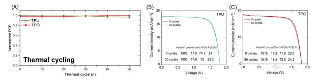
Fig. 5 (A) Power conversion efficiency trend during 50 cycles of TC test. (B) and (C) Comparison between the J-V curves before and after the TC test in the case of two minimodules encapsulated with TPU and TPO, respectively.
