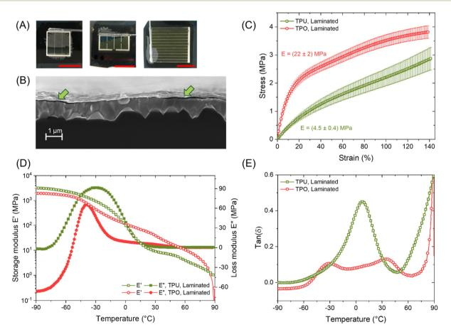
Fig. 4 (A) Macroscopic delamination observed on different tandem layouts with different sizes. Red bar: 1 cm. (B) Microscopic delamination observed *via* a cross-sectional scanning electron microscopy image of the tandem solar cell. For vacuum-laminated (cured) samples of TPU and TPO: (C) Stress–strain curves. (D) Storage and loss moduli as a function of temperature. (E) tan(δ) as a function of temperature.
