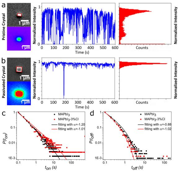
Fig. 3 SEM and PL images, PL intensity time trajectories (10 min, 100 ms bin time) and corresponding histograms of single MAPbI<sub>3</sub> crystals (a) before and (b) after the 3% MACI post-treatment, respectively. In the PL images, purple to red colors based on the rainbow sequence represent gradually higher intensities. Normalized probability distributions of the duration of (c) ON times and (d) OFF times of MAPbl<sub>3</sub> NCs with 0, 3%Cl surface treatment.
