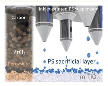
Fig. 1 Conceptual illustration depicting an inkjet-printing process of a sacrificial layer of polystyrene (PS) particles for nano-architectured perovskite solar cells with carbon-based electrodes with a solar cell structure depicted on the left.
