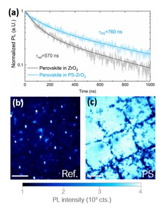
Fig. 3 (a) Time-resolved photoluminescence (TRPL) measurements of the perovskite embedded in reference  $ZrO_2$  and nano-architectured  $ZrO_2$  (PS- $ZrO_2$ ), showing a difference in the decay constant and charge-carrier lifetime. Steady-state PL maps of (b) reference perovskite solar cells with carbon electrodes and (c) nano-architectured cells with a PS sacrificial layer. Scale bar  $-150~\mu m$ .
