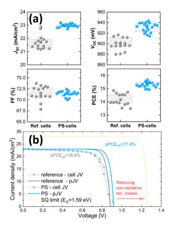
Fig. 4 (a) Short-circuit current density  $(J_{SC})$ , open-circuit voltage  $(V_{OC})$ , fill factor (FF) and power conversion efficiencies of manufactured CPSCs with and without a sacrificial PS laver. (b) JV curves and pseudo-JV curves of the optimum reference and nano-architectured cells, in comparison with the curve at the Shockley-Queisser limit.
