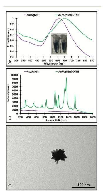
**Fig. 2** UV-Visible spectra and photograph of the solution (A), SERS spectra (B) of the Au/AgNSs and Au/AgNSs@DTNB; and the TEM image (C) of the Au/AgNSs.
