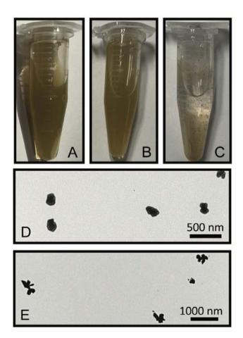
Fig. 7 Photographs of the nanotags (A), nanosupernova (B) and the Au/ AgNSs@Ag particles (C). The nanotags and nanosupernova are stable in solution, however when no DTNB is added the particles aggregate. TEM images of particles made using the synthesis method for nanotags (D) and nanosupernova (E), but without the addition of hydroquinone.
