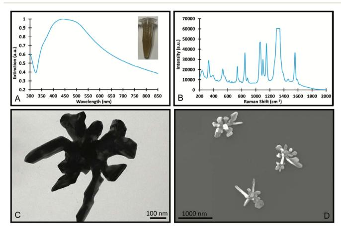
Fig. 5 UV-Visible spectrum (A), SERS spectrum (B), TEM Image (C) and SEM images (D) of the SERS nanosupernova formed with 90 µL of 10 mM AgNO<sub>3</sub> and 30  $\mu$ L of hydroquinone and incubated for 12 h.
