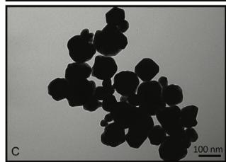
Fig. 3 UV-Visible spectrum and the photograph of the solution (A), SERS spectrum (B) and TEM Image (C) of the SERS nanotags formed with 90  $\mu L$  of 10 mM AgNO $_3$  and 30  $\mu L$  of hydroquinone and incubated for 1 h.
