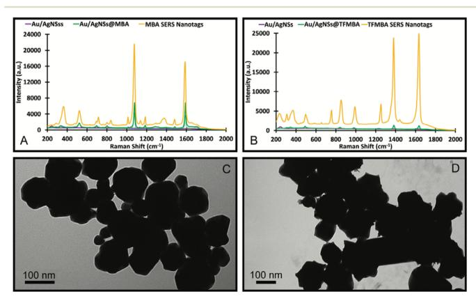
Fig. 8 SERS spectra of the MBA SERS nanotags (A) and TFMBA SERS nanotags (B) made with 30 μL AgNO3 and 30 μL hydroquinone then incubated for 12 hours. The figure includes TEM images of the MBA nanotags (C) and TFMBA nanotags (D).
