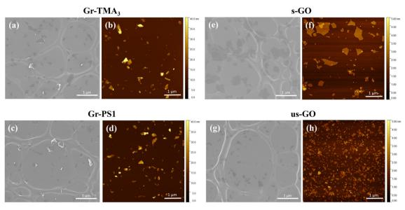
Fig. 1 Physicochemical characterisation of (a and b) Gr-TMA<sub>3</sub>, (c and d) Gr-PS1, (e and f) s-GO and (g and h) us-GO: (a, c, e and g) electron and (b, d, f and h) AFM micrographs were obtained for lateral dimension and thickness measurements, respectively.
