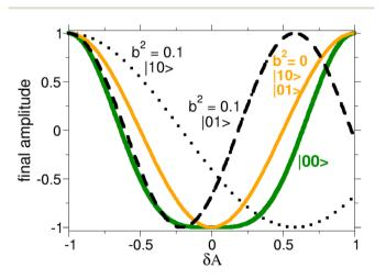
Fig. 2 Dependence of the final amplitude of the starting state (|00),  $|01\rangle$  and  $|10\rangle$ ) on deviations from  $\pi$  in the pulse areas of odd pulses  $(\delta A_1 = \delta A_3 = \delta A)$ , and of  $2\pi$  in the second pulse  $(\delta A_2 = 2\delta A)$ , for different geometrical factors.
