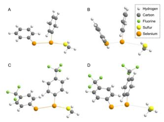
Fig. 7 Optimized geometries of TCI (A) and (C) and TS (B) and (D) from (PhSe)<sub>2</sub> (A), (B) and (CF<sub>3</sub>PhSe)<sub>2</sub> (C), (D), respectively. Molecules are represented by the ball-and-stick model, colour code H: white, C: grey, F: green and Se: orange. Level of theory: (COSMO)-ZORA-OLYP/TZ2P.
