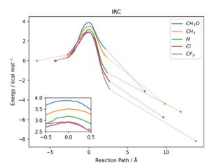
Fig. 8 IRC profiles of the investigated reactions in water. The dashed lines represent the path between the last computed IRC point and the geometry optimized structures of reactants and products (colored diamonds). The TS region is shown in more detail in the inset. Level of theory COSMO-ZORA-OLYP/TZ2P
