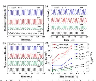
Fig. 5 Time-dependent photocurrent density of NbSe<sub>2</sub>/Nb<sub>2</sub>O<sub>5</sub> under the different centrifugal speed (1000, 3000, 5000, and 7000 rpm)-based PEC photodetectors was measured at (a) 0.2 V, (b) 0.4 V, and (c) 0.6 V; (d)  $I_{\rm ph}$ and  $R_{ph}$  values of the 2D material-based PEC-type photodetector, including NbSe<sub>2</sub>/Nb<sub>2</sub>O<sub>5</sub> (this work), BP, 41 InSe, 43 and Te. 42
