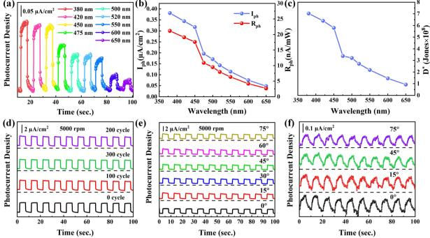
Fig. 8 (a) Photocurrent density, (b) the calculated Iph and Rph, and (c) specific detectivity (D\*) values under different wavelengths; flexibility measurement with (d) different bending cycles and (e) bending angles in the PEC-type photodetector; (f) flexibility measurement in various bending angles in a solid photodetector
