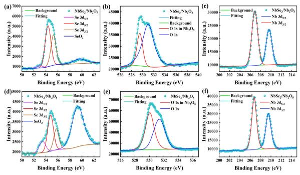
Fig. 4 XPS signal of bulk NbSe<sub>2</sub> with (a) Se, (b) O, and (c) Nb elements; XPS signal of NbSe<sub>2</sub>/Nb<sub>2</sub>O<sub>5</sub> nanosheets with (d) Se, (e) O, and (f) Nb elements.
