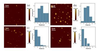
Fig. 3 AFM images and statistical size distribution of few-layer NbSe<sub>2</sub>/ Nb<sub>2</sub>O<sub>5</sub> nanosheets under the centrifugation speed of (a) 1000 rpm, (b) 3000 rpm, (c) 5000 rpm, and (d) 7000 rpm.
