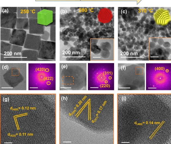
Fig. 2 (a-c) TEM images of NaSbS<sub>2</sub> NCs formed at 250, 280 and 310 °C, respectively the scale bar in the inset images is 50 nm. (d-f) are the magnified images (scale bar is 50 nm) and FFT patterns. (g-i) magnified images of NaSbS<sub>2</sub> NCs. The scale in panels (g-i) is 5 nm respectively.
