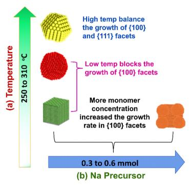
Fig. 3 Schematic of the controlled synthesis of NaSbS<sub>2</sub> for different reaction parameters (a) reaction temperature and (b) Na precursor molar ratio.
