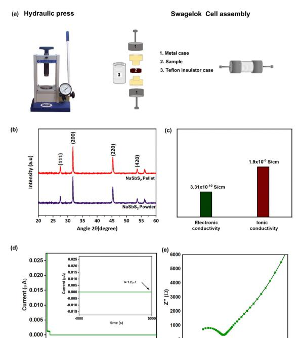
Fig. 6 (a) Schematic for Swagelok cell assembling (b) XRD pattern of the pellet and powder NaSbS<sub>2</sub> before and after cold press (c) bar graph of electronic and ionic conductivity (d) DC polarization of NaSbS2 with inset showing the current behaviour for duration of 5000 s (e) Nyquist plot of Electrochemical Impedance Spectroscopy (EIS) of NaSbS<sub>2</sub> pellet.
