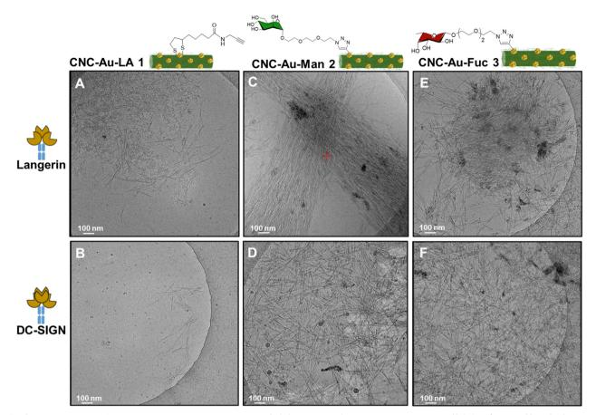
Fig. 3 Cryo-TEM images of the chimera lectins langerin-Fc and DC-SIGN-Fc in TMS treated with a dispersion (0.01% w/w in  $H_2O$ ) of CNC-Au-LA **1** (A and B), respectively; or CNC-Au-Man **2** (C and D), respectively; or CNC-Au-Fuc **3** (E and F), respectively. Chimera lectins were used at the final concentration of 0.1 mg mL<sup>-1</sup> (ESI†). Buffer TMS: 20 mM TRIS, 150 mM NaCl, 1.0 mM CaCl<sub>2</sub>, 2.0 mM MgCl<sub>2</sub>, pH = 8. Scale bar 100 nm.
