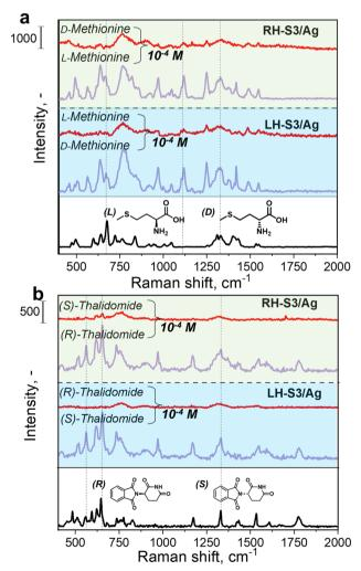
Fig. 4 (a) Stacked SERS spectra of  $10^{-4}$  M L/D-methionine enantiomer deposited on LH- or RH-S3/Ag substrates from methanol solutions measured at 785 nm, (b) SERS spectra of  $10^{-4}$  M (R)/(S)-thalidomide enantiomer deposited on LH- or RH-S3/Ag substrates from methanol solutions measured at 780 nm measured at 785 nm. Bottom spectra (black) show Raman spectra of both compounds
