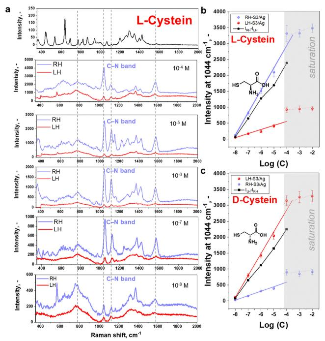
Fig. 2 (a) Stacked SERS spectra of L-cysteine enantiomer deposited on LH- or RH-S3/Ag substrates from methanol solutions with various initial concentrations (10<sup>-4</sup>-10<sup>-8</sup> M range) measured at 785 nm; (b) and (c) the characteristic L-cysteine and D-cysteine SERS band (1044 cm<sup>-1</sup>) intensity as a function of the initial enantiomers concentrations and plasmonic substrate LH- or RH-kind.
