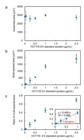
Fig. 2 Calibration curve of HCT116 standard nanoscale EVs for lightinduced acceleration in a microchannel. (a) Assembly area, (b) multilayered area, and (c) ratio of the multi-layered area at each concentration of EV standard. Inset: Low concentration range. Error bars are standard deviations (n = 3).
