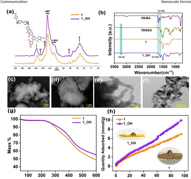
Fig. 1 (a) <sup>13</sup>C-CPMAS spectra of 1 and 1\_OH; (b) IR spectra of TRIRES, VBrBA, 1, and 1\_OH; (c and d) FESEM images of 1 and 1\_OH; (e and f) HRTEM images of 1 and 1\_OH; (g) thermogravimetric analysis of 1 and 1\_OH under N<sub>2</sub> atmosphere at a ramp rate of 5 °C min<sup>-1</sup>; and (h) water adsorption isotherms of 1 and 1\_OH with insets presenting photographs from the contact angle measurements.
