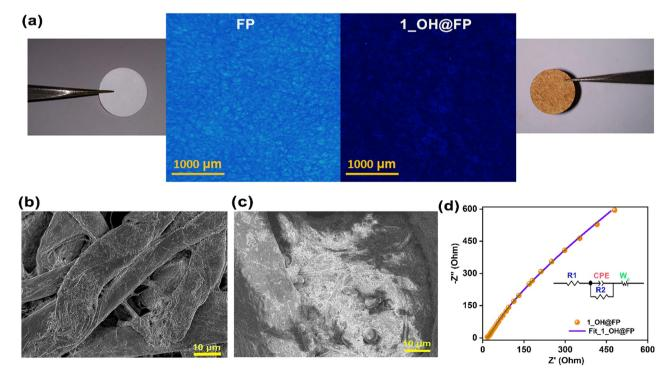
Fig. 3 (a) Macro zoom fluorescence microscope images of neat FP and 1\_OH@FP with the corresponding photographs on the side. (b, c) FESEM image of neat FP and 1\_OH@FP. (d) Equivalent circuit fit to the Nyquist plot of 1\_OH@FP at 80 °C and 95% RH.
