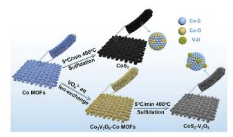
Fig. 1 Schematic illustration of the synthesis strategy of CoS<sub>2</sub> and CoS<sub>2</sub>- $V_2O_5$  nanoarrays supported on carbon cloth (CC).
