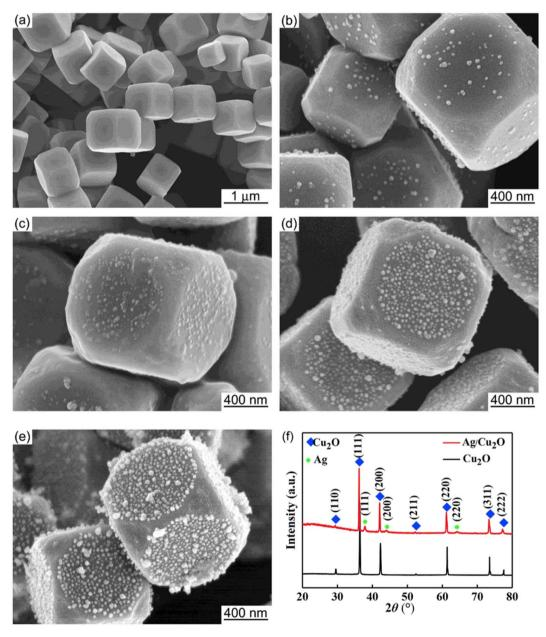
Fig. 2 SEM images of (a) pristine  $Cu_2O$  and (b-e) Ag-decorated  $Cu_2O$  nanostructures, representing a core-satellite structure. The number of Ag satellites increased with increasing concentration of AgNO<sub>3</sub> (from (b) to (e)). The XRD patterns for (a) and (e) are shown in (f). Reproduced with permission from ref. 38. Copyright 2019 Elsevier.
