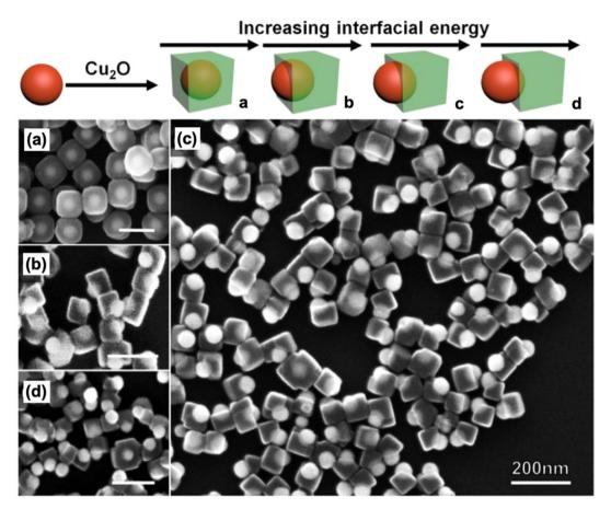
Fig. 6 Schematic illustration of the tunable synthesis of Janus-type Au−Cu<sub>2</sub>O nanocomposites through control of interfacial energy using AMBI as the modifying ligand. Also shown are the SEM images of the structures obtained (a) without AMBI and (b-d) with increasing AMBI concentration. Reproduced with permission from ref. 87. Copyright 2020 Wiley-VCH.
