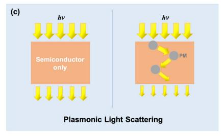
Fig. 10 Schematic depiction of the three primary mechanisms for plasmon-enhanced photocatalysis by plasmonic metal-semiconductor nanocomposites: (a) hot electron injection (HEI), (b) plasmon-induced near-field interaction, and (c) plasmonic light scattering.
