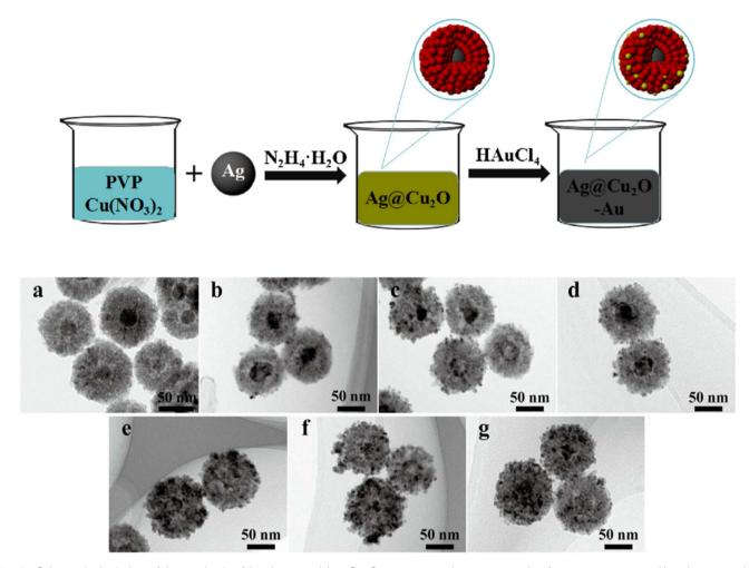
Fig. 8 Schematic depiction of the synthesis of Au-decorated Ag@Cu<sub>2</sub>O nanocomposites, an example of a ternary structure. Also shown are the TEM images of the structures obtained (a) without Au and (b-g) with increasing loading amount of Au. Reproduced with permission from ref. 95. Copyright 2018 Elsevier.
