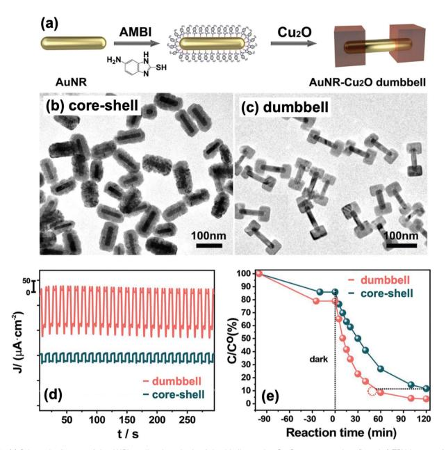
Fig. 7 (a) Schematic diagram of the AMBI-mediated synthesis of dumbbell-type  $Au-Cu_2O$  nanocomposites. (b and c) TEM images of the structures obtained (b) without AMBI and (c) in the presence of AMBI. (d and e) Comparison of the (d) photocurrent response and (e) photocatalytic activity for MO degradation of dumbbell and core-shell structures. Reproduced with permission from ref. 92. Copyright 2023 Wiley-VCH.
