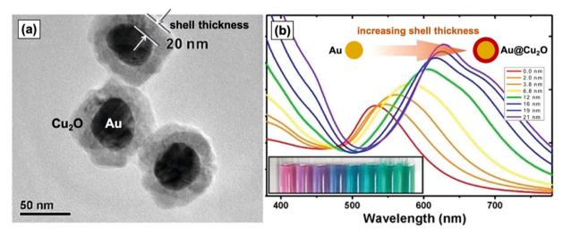
Fig. 1 (a) TEM image of Au-Cu<sub>2</sub>O nanocomposites with a core-shell structure. (b) UV-vis spectra and photograph (inset) of colloidal dispersions of Au-Cu<sub>2</sub>O core-shell nanocomposites with increasing Cu<sub>2</sub>O shell thickness (from left to right), clearly showing the redshifting of the LSPR band. Reproduced with permission from ref. 36. Copyright 2012 American Chemical Society.
