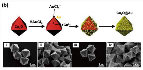
Fig. 4 Schematic depiction of the formation of (a)  $Cu_2O@Ag$  and (b)  $Cu_2O@Au$  core—shell nanocomposites through GRR. Also shown are the SEM images of the structures produced with (i) no metal and ((ii) to (iv)) increasing loading amount of metal. Reproduced with permission from (a) ref. 69, copyright 2017 the Royal Society of Chemistry, and (b) ref. 62, copyright 2016 Elsevier.
