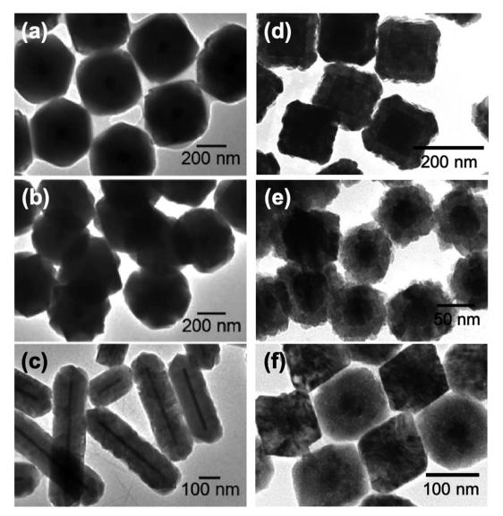
Fig. 3 TEM images of (a-c) Au@Cu2O and (d-f) Ag@Cu2O core-shell nanocomposites with different morphologies. Reproduced with permission from (a-c) ref. 50, copyright 2009 American Chemical Society, and (d-f) ref. 49, copyright 2014 American Chemical Society.
