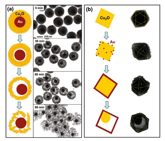
Fig. 5 Schematic representation of the formation of (a)  $Au@Cu_2O$  and (b)  $Cu_2O@Au$  yolk—shell nanocomposites. The TEM images of the structures produced are also shown. Adapted with permission from (a) ref. 80, copyright 2011 American Chemical Society, and (b) ref. 84, copyright 2017 Springer Nature.
