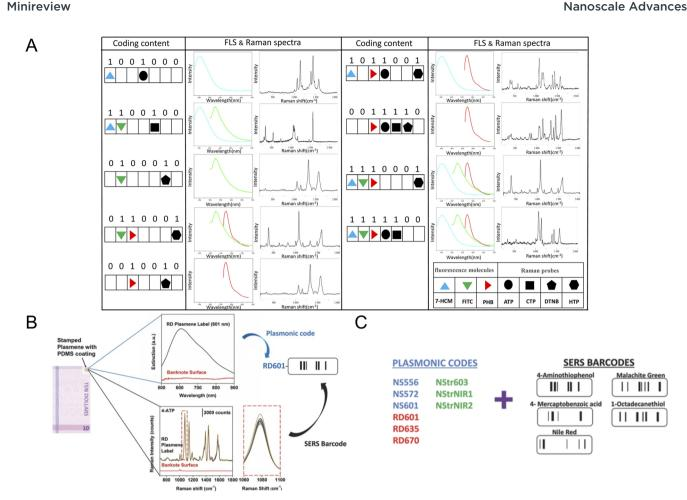
Fig. 8 (A) Raman-fluorescence combined encoding for security labels; Raman-absorption combined encoding for security labels. Reproduced with permission from ref. 60. Copyright 2016 American Chemical Society. (B) Schematic diagram of the encoding source; (C) double layer encoding – plasmonic encoding and Raman encoding. Reproduced with permission from ref. 61. Copyright 2015 John Wiley & Sons, Inc.
