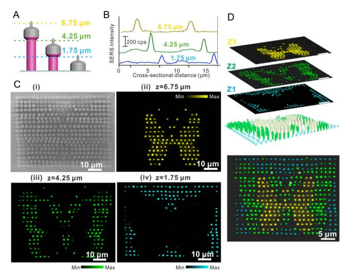
Fig. 5 Three-dimensional micro-candlestick for a security label. (A) Schematic diagram of the three-dimensional micro-candlestick; (B) corresponding Raman spectra; (C) scanning electron microscopy (SEM) images and Raman imaging images of different heights of the threedimensional micro-candlestick; (D) schematic diagram of the three-dimensional micro-candlestick forming patterns at different scan heights. Reproduced with permission from ref. 56. Copyright 2017 American Chemical Society.
