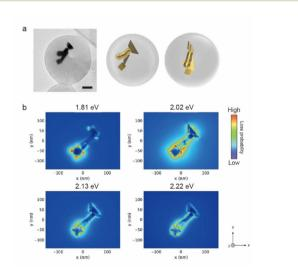
Fig. 5 (a) TEM image of gold NPs encapsulated in a silica nanocapsule under light illumination and the proposed model structures of the welded three AuNTs observed in the TEM image. Scale bar is 50 nm. (b) EEL maps of the welded gold nanostructure in (a).
