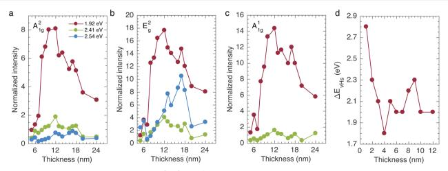
Fig. 3 (a-c) Intensity normalized by silicon peak of  $A_{1g}^2$ ,  $E_g^2$ , and  $A_{1g}^1$  modes as a function of QL thickness for excitation laser energies of 1.92 eV, 2.41 eV, and 2.54 eV, respectively. (d) The energy difference calculated between van Hove singularities (vHs) from 1 to 12 QLs.
