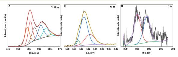
Fig. 4 High-resolution fitted XPS spectra of (a) Ni 2p<sub>3/2</sub>, (b) O 1s, and (c) C 1s for MAS-N70.
