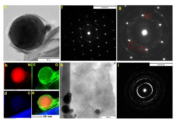
Fig. 2 (a) TEM image, (b—e) EDS mapping, (f) corresponding SAED pattern, (g) zoomed-in region of the SAED pattern, (h) TEM image of nanosheets, and (i) corresponding SAED pattern.
