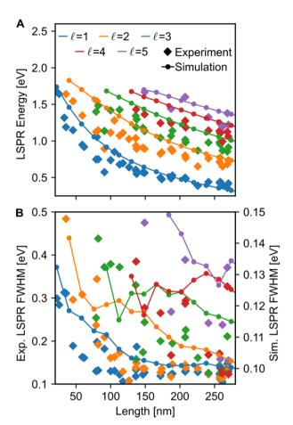
Fig. 4 Length effect on the resonances of Cu NRs. (A) Energies and (B) FWHMs of the color-coded longitudinal LSPRs. The diamonds are experimental values and the connected dots are numerical simulations for 12 nm wide NRs. In (B), the left y-axis corresponds to the experimental data, and the right y-axis corresponds to the simulated data.
