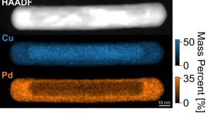
Fig. 1 Shape and composition of Cu and Cu–CuPd NRs. TEM image of representative (A) Cu NRs and Cu–CuPd NRs with varying concentrations of Pd precursor resulting in NRs with Pd mass percent of (B) 22, (C) 42, and (D) 46%. (E) HAADF signal and STEM-EDS elemental maps for Cu and Pd in a Cu–CuPd NR from the batch containing 46% Pd by mass.
