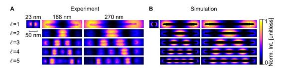
Fig. 3 Longitudinal LSP mode excitation distribution in Cu NRs. (A) STEM-EELS NMF spatial loadings (experiment) and (B) EEL probability maps (simulation) at different energies for the  $\ell=1-5$  LSP modes of three representative Cu NRs of labelled length and width of 12–13 nm.
