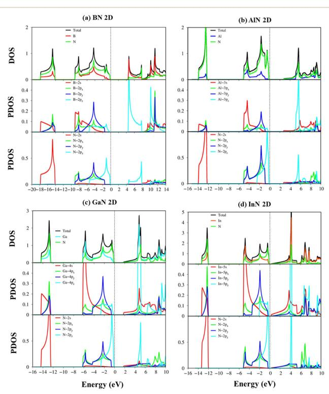
Fig. 7 (a-d) Van Hove singularities of the density of states (DOS) and project-density of states (PDOS) of the BN, AIN, GaN, and InN monolayers, respectively, and those coming from B-/Al-/Ga-/In-/N- orbitals (red, blue, cyan, yellow, and green curves), as well as B-(2s, 2px, 2py, and 2pz), Al- $(3s, 3p_x, 3p_y, and 3p_z)$ ,  $Ga-(4s, 4p_x, 4p_y, and 4p_z)$ ,  $In-(5s, 5p_x, 5p_y, and 5p_z)$ , and  $N-(2s, 2p_x, 2p_y, and 2p_z)$  orbitals (red, green, blue and cyan curves).
