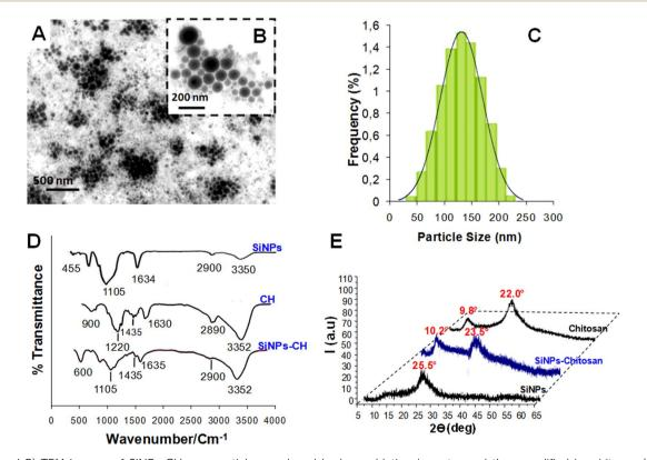
Fig. 1 (A and B) TEM images of SINPs-CH nanoparticles produced by laser ablation in water and then modified by chitosan (CH). (B) is a magnification of (A). (C) Particle-size distribution of the chitosan-coated nanoparticles (SiNPs-CH) determined by a Zetasizer Nano ZS instrument (DLS). (D) FTIR spectra of chitosan, SiNPs, and SiNPs-CH. (E) XRD patterns of SiNPs-CH compared to those of chitosan and uncoated SiNPs.
