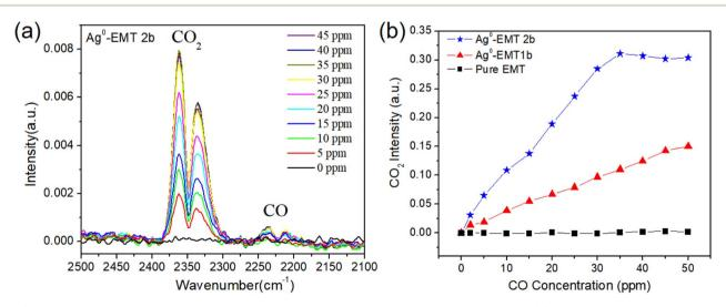
Fig. 4 (a) In situ IR spectra Ag-EMT-2b film by increasing the CO concentration from 2 to 50 ppm at RT. (b) The IR absorption intensities of CO<sub>2</sub> dependent on the amount of CO with pure EMT, Ag-EMT-1b, and Ag-EMT-2b films in the range of 2–50 ppm.
