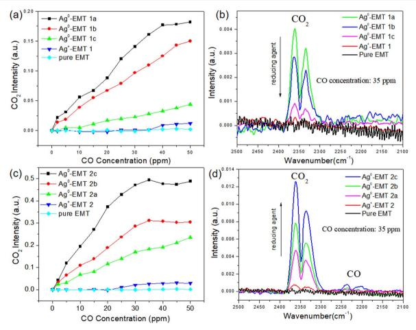
Fig. 5 (a) The  $CO_2$  intensities dependent on CO with unreduced  $Ag^+$ -EMT 1 sample and reduced Ag-EMT 1a, 1b, and 1c samples with different amounts of reducing agent and (b) the corresponding *in situ* IR spectra measured. (c) The  $CO_2$  intensities dependent on CO with unreduced  $Ag^+$ -EMT 2 sample and reduced Ag-EMT 2a, 2b, and 2c samples and (d) the corresponding *in situ* IR spectra measured.
