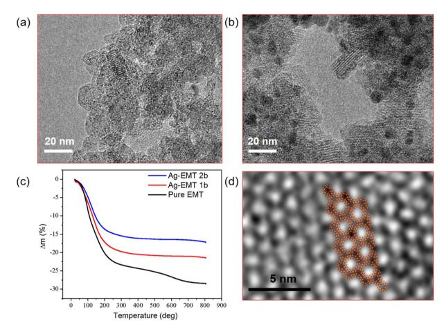
Fig. 2 TEM images of (a) Ag-EMT 1b and (b) Ag-EMT 2b and (insets) corresponding EDX analysis. (c) TG curves of pure EMT, Ag<sup>0</sup>-EMT 1b, and Ag<sup>0</sup>-EMT 2b samples. (d) Enlarged TEM images of Ag-EMT zeolite and the schematic diagram of EMT framework structure.
