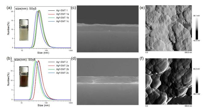
Fig. 3 Particle size distribution curves of the (a) Ag-EMT 1 and (b) Ag-EMT 2 samples. The average size of the nanoparticles is  $50 \pm 5$  nm. The insets are coating suspensions of Ag-EMT 1b and Ag-EMT 2b, respectively. (c) and (d) are the SEM images of Ag-EMT films of Ag-EMT 1b and Ag-EMT 2b, and the thickness is 500 nm. The scale bar is 2  $\mu$ m. (e) and (f) are the AFM images of the Ag-EMT films of Ag-EMT 1b and Ag-EMT 2b.
