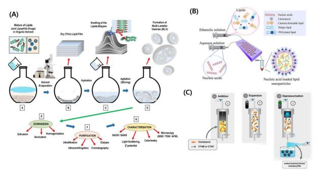
Fig. 1 (A) Schematic illustration of the conventional nanovesicle formulation method. Reproduced with permission (Lombardo *et al.* 2020) from MDPI.<sup>217</sup> (B) Schematic illustration of the microfluidic approach.<sup>218</sup> Reproduced with permission (Ali *et al.* 2021) from American Chemical Society.<sup>218</sup> (C) Schematic illustration of compressed fluid-based methods.<sup>50</sup> Reproduced with permission (Ballell-Hosa *et al.* 2022) from MDPI.<sup>50</sup>
