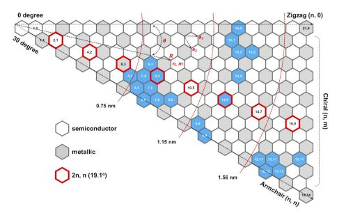
Fig. 2 Semiconducting and metallic SWNT species: (n,m) SWCNTs (blue hexagon) achieved so far by direct chirality selection synthesis.<sup>24</sup>
