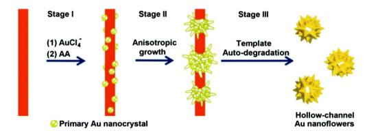
Fig. 5 Schematic illustration of the proposed mechanism for the formation of hollow gold nanoflowers: stage (II) Au nucleates on the template surface; stage (III) Au primary crystal undergoes anisotropic growth to form branches; stage (III) the as-formed Au nanoflowers catalyze the degradation of the template in the presence of AA, leaving the open hollow channel and releasing the individual HAuNFs. Adapted with permission from ref. 130. Copyright © The Royal Society of Chemistry 2016.
