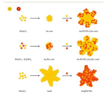
Scheme 5 Schematic illustration of the formation of three morphology-controlled Au–Pd nanoflowers (Au–Pd NFs) by seed-mediated growth. Adapted with permission from ref. 336. Published by MDPI. Copyright@ 2017 by Tao Ma et al.
