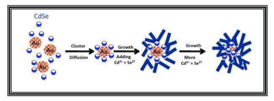
Scheme 1 Proposed mechanism for the formation of the Au@CdSe nanoflowers. Reprinted with permission from ref. 128. Copyright © 2011 WILEY-VCH Verlag GmbH & Co. KGaA, Weinheim.
