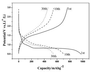
Fig. 19 The first (solid line), 10th (dashed line), and 30th (dotted line) charge—discharge curves of flower-like  $\alpha$ -Fe<sub>2</sub>O<sub>3</sub> nanostructures at a current density of 0.2 mA cm<sup>-2</sup>. Reprinted with permission from ref. 306. Copyright © 2008, American Chemical Society. All rights reserved.
