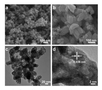
Fig. 15 SEM (a and b), TEM (c), and HR-TEM (d) images of the hnp– ${\rm Pt}_{35}{\rm Cu}_{65}$  alloy. Reprinted with permission from ref. 354. Copyright © 2017 Elsevier Inc.
