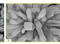
Fig. 10 FE-SEM images of CuO nanoflowers prepared at 170 °C for 24 h with different magnifications of: (a)  $10000 \times$ , (b)  $20000 \times$ , and (c) 1000 00×. Reprinted with permission from ref. 129. Copyright © 2014 Elsevier Ltd. All rights reserved.
