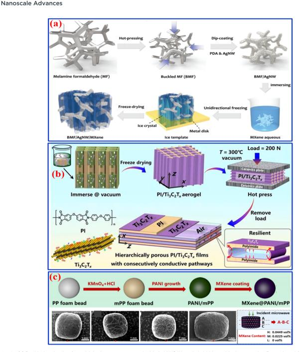
Fig. 8 (a) Buckled melamine formaldehyde sponges coated with AgNW/MXene hybrid hierarchical composite. Reproduced from ref. 148 with permission from the Royal Society of Chemistry, © 2019. (b) Hierarchically porous PI/Ti<sub>3</sub>C<sub>2</sub>T<sub>x</sub> composite. Reproduced from ref. 108 with permission from the Authors, © 2021. (c) MXene network decorated with polypropylene foam beads. Reproduced from ref. 149 with permission from Elsevier Ltd., © 2020.
