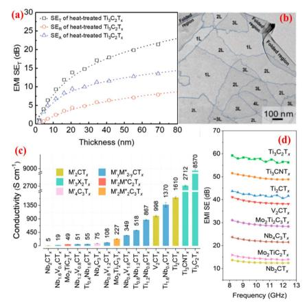
Fig. 2 (a) EMI SE values of  $Ti_3C_2T_x$  film after annealing at 400 °C and (b) transmission electron microscopy image of few-layer thick MXene film. Reproduced with permission from ref. 62 with permission from Wiley-VCH Verlag GmbH & Co. KGaA, Weinheim, © 2020. (c) Conductivity and (d) EMI SE of 5 μm-thick MXene films with different compositions. Reproduced from ref. 63 with permission from the American Chemical Society, © 2020.
