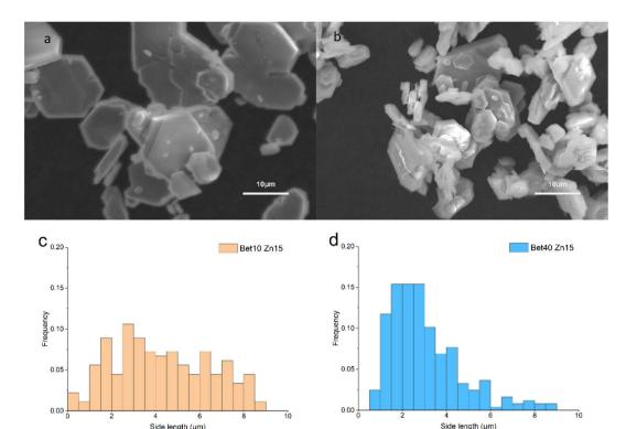
Fig. 10 SEM images (a and b) for simonkolleite synthesized, after 15 days, and the size distribution of the side lengths (n = 200 hexagonal crystals) (c and d) for 10% of betaine (a and c) and 40% of betaine (b and d).
