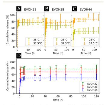
Fig. 6 Drug release kinetics of ibuprofen at 25  $^{\circ}$ C and 37.5  $^{\circ}$ C for (A) EVOH32, (B) EVOH38 and (C) EVOH44. (D) Influence of the ethylene content on the release of ibuprofen at 25  $^{\circ}$ C. The curves were fitted with a desorption model according to eqn (5).
