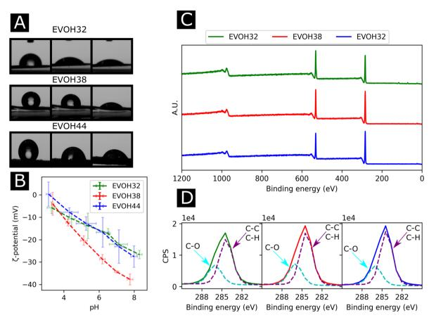
Fig. 3 (A) Images of the sessile drop measurement at 1 s, 30 s and 90 s (from left to right), (B) surface  $\zeta$ -potential from pH 3 to pH 9, (C) X-ray photoelectron spectroscopy survey scans of the membranes and (D) region scan for the C 1s environment for each EVOH copolymer.
