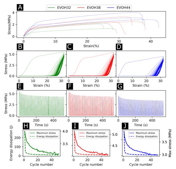
(A) Stress-strain curves for the three EVOH electrospun membranes. Stress over strain of quasi-static cyclic tensile testing for 50 cycles for (B) EVOH32, (C) EVOH38 and (D) EVOH44 (average of three independent samples). Stress over time for (E) EVOH32, (F) EVOH38 and (G) EVOH44 for 50 cycles (examples of single specimens). Energy dissipation and maximum stress for (H) EVOH32, (I) EVOH38 and (J) EVOH44 for each cycle (average of three independent samples).
