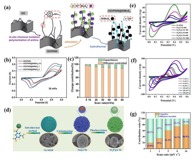
Fig. 4 (a) Preparation process schematic of rGO/PANI@NiMoS4, (b) CV curves at varying scan rates, (c) charge involvement of rGO/ PANI@NiMoS<sub>4</sub>, (d) preparation process schematic of Ni<sub>2</sub>P@CM, a nanoscale nickel phosphide encapsulated in a carbon microsphere, (e) comparison of CV curves of composites, (f) CV curves of Ni<sub>2</sub>P@CM-900 at scan rates ranging from 1 mV s<sup>-1</sup> to 30 mV s<sup>-1</sup>, and (g) specific capacitance of composites
