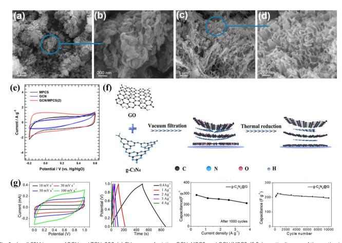
Fig. 8 (a–d) SEM images of BCN and TCN-200. (e) CV curves of pristine GCN, MPCS, and GCN/MPCS. (f) Schematic diagram of the synthesis of the graphene/g- $C_3N_4$  composite, and (g) CV, GCD curves and corresponding capacitance value.
