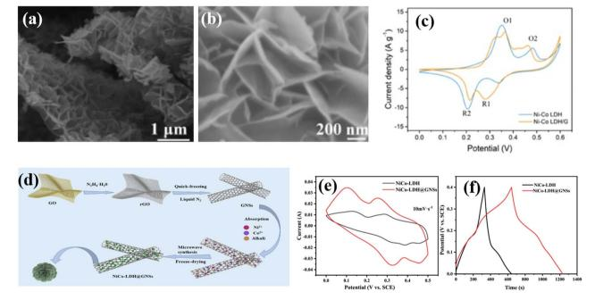
Fig. 7 (a) Low and (b) high magnification SEM images of the Ni-Co LDH/G composite, (c) a comparison of CV curves, (d) a schematic of the synthesis process of NiCo-LDH@GNSs, (e) CV curves of both pristine NiCo-LDH and NiCo-LDH@GNSs, and (f) CV curves of activated carbon and the NiCo-LDH@GNS composite at a scan rate of 10 mV s<sup>-1</sup>.
