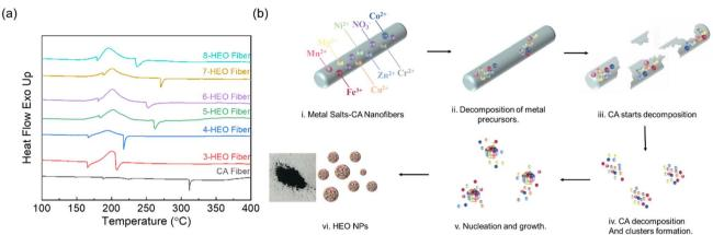
Fig. 2 (a) DSC of the fibers, and (b) proposed mechanism of HEO nanoparticles formation by converting the electrospun nanofibers *via* low-temperature annealing in air and the accomplished powder. A digital photograph of the as-synthesized HEO NPs.
