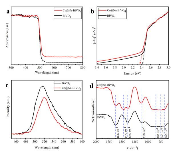
Fig. 5 (a) UV-vis/DRS, (b) energy diagram, (c) PL spectra (both catalysts at the same concentration in ethanol) and (d) FT-IR spectra of the assynthesized  $BiVO_4$  and  $Co@Na-BiVO_4$  (powders compressed into KBr pellets).
