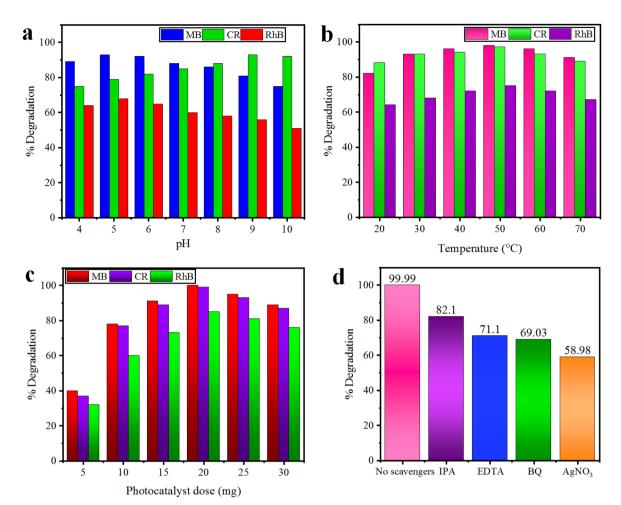
Fig. 9 Effect of (a) pH, (b) temperature and (c) photocatalyst dose on MB, CR, and RhB dyes using the Co@Na-BiVO<sub>4</sub> catalyst, whereas (d) represents the role of major active species.
