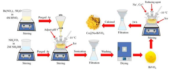
Fig. 1 Scheme employed for the synthesis of BiVO<sub>4</sub> and Co@Na-BiVO<sub>4</sub>.
