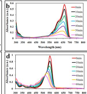
Fig. 6 UV-vis spectrophotometry results: (a) lambda max, (b) MB, (c) CR and (d) RhB obtained over Co@Na-BiVO<sub>4</sub> photocatalysts.
