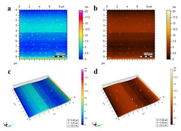
Fig. 4 AFM images of Co@Na-BiVO<sub>4</sub> (a and b) topographical images, and (c and d) three-dimensional view.
