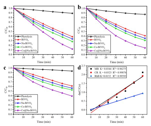
Fig. 7 Comparative degradation activities of dyes with photolysis (degradation via photons), BiVO<sub>4</sub>, Na-BiVO<sub>4</sub>, Co-BiVO<sub>4</sub> and Co@Na-BiVO<sub>4</sub> (a) MB, (b) CR and (c) RhB, whereas (d) represents the kinetic study for MB, CR and RhB obtained over Co@Na-BiVO<sub>4</sub> photocatalysts.
