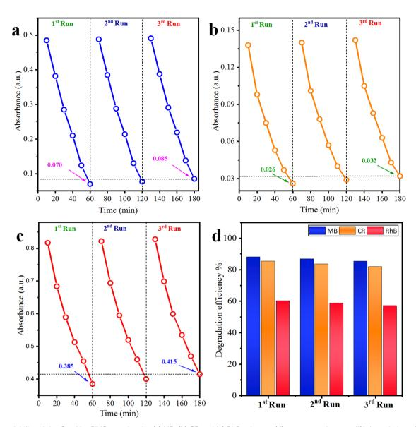
Recyclability of the Co@Na-BiVO<sub>4</sub> catalyst for (a) MB, (b) CR and (c) RhB, whereas (d) represents the overall% degradation efficiency.
