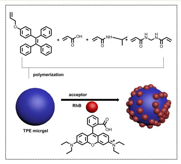
Fig. 9 Schematic illustration of the construction of a temperature and pH responsive nano-ALHS based on synthetic AIE-active microgels with TPE AlEgens. Reproduced with permission from ref. 108. Copyright 2021, Wiley-VCH.
