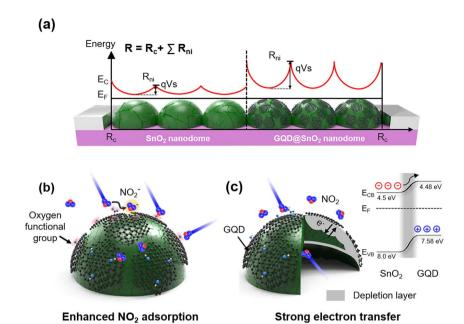
Fig. 5 Schematic illustration for (A) initial potential barrier formation for the SnO<sub>2</sub> nanodomes structure. (B and C) Schematic illustration of the NO<sub>2</sub> sensing mechanism for GQD@SnO<sub>2</sub> nanodomes showing (B) enhanced NO<sub>2</sub> adsorption due to the GQDs and (C) formation of an electron depletion layer with its electronic band structure.
