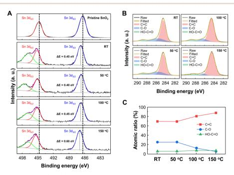
Fig. 4 X-ray photoelectron spectroscopy (XPS) (A) Sn 3d and (B) C 1s spectra of pristine SnO₂ nanodomes and GQD@SnO₂ nanodomes prepared at various annealing temperatures. (C) Atomic ratio of carbon bonds as a function of annealing temperature.
