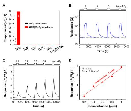
Fig. 3 (A) Selective NO<sub>2</sub> gas sensing performance of GQD@SnO<sub>2</sub> nanodome based gas sensors. (B) Resistance curve of GQD@SnO<sub>2</sub> to 5 ppm  $NO_2$  with repeated exposure. (C) Response curves to different  $NO_2$  concentrations under a 1 ppm concentration. (D) Linear fit of the responses as a function of NO<sub>2</sub> concentration.
