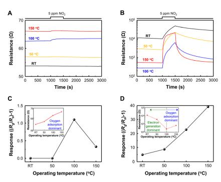
Fig. 2 Resistance curves for 5 ppm NO<sub>2</sub> as a function of operating temperature for (A) pristine SnO<sub>2</sub> nanodomes and (B) a GQD@SnO<sub>2</sub> nanodome based gas sensor. Gas response for (C) pristine SnO<sub>2</sub> nanodomes and (D) a GQD@SnO<sub>2</sub> nanodome based gas sensor. The insets of (C and D) represent the base resistance as a function of operating temperature.
