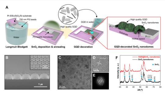
Fig. 1 Fabrication and characterization of GQD-decorated  $SnO_2$  (GQD@ $SnO_2$ ). (A) Schematic illustration of the fabrication process for a GQD@ $SnO_2$  nanodome based gas sensor. (B) Cross-sectional SEM image of GQD@ $SnO_2$  nanodomes. The inset shows a plain-view SEM image of GQD@ $SnO_2$  nanodomes. (C) HR-TEM image of GQD@ $SnO_2$  nanodomes, (D) lattice fringe images, and (E) FFT of the GQDs. (F) XRD patterns of  $SnO_2$  nanodomes and GQD@ $SnO_2$  nanodomes.
