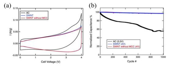
Fig. 6 (a) Cyclic voltammetry curves of AC, SWCNTs, and SWCNTs without MCC measured at  $1 \text{ mV s}^{-1}$  and (b) cycle stability over 1000 cycles at  $1 \text{ A g}^{-1.51}$  [This figure has been adapted/reproduced from ref. 51 with permission from John Wiley and Sons, copyright 2010.]
