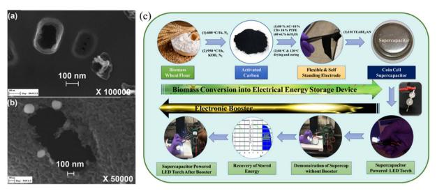
Fig. 4 (a) and (b) SEM images of activated carbon by  $CO_2$  activation at 800 °C and by  $H_2O$  activation at 700 °C<sup>42</sup> and (c) schematic representation of conversion of wheat flour into a high energy density supercapacitor electrode with an additional booster circuit for the recovery of stored energy as a proof of concept.44 [This figure has been adapted/reproduced from ref. 42 and ref. 44 with permission from Elsevier, copyright 2018 and from John Wiley and Sons, copyright 2020.]
