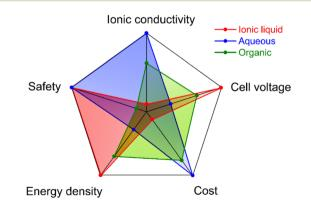
Fig. 3 Comparison of the properties and performance of IL, aqueous, and organic electrolytes. Reproduced from ref. 14 [this figure has been adapted/reproduced from ref. 14 with permission from the Royal Society of Chemistry, copyright 2021].
