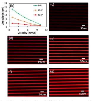
(a) Schematic illustration of the EHD printing system comprising a single nozzle, a movable platform, a conductive platform and a power supply system, (b) and (c-g) fluorescence images of patterned lines with QD ink of 6 cP at printing speeds of 10 mm  $s^{-1}$ , 7 mm  $s^{-1}$ , 5 mm s<sup>-1</sup>, 3 mm s<sup>-1</sup> and 1 mm s<sup>-1</sup>, respectively.
