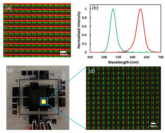
Fig. 5 (a) Magnified photoluminescence images of the two-color (red and green) bottom-emission QLED devices, (b) EL emission spectra of red and green sub-pixels, (c) the photo and (d) the magnified electroluminescence images of red and green sub-pixels when lightening simultaneously.
