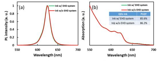
Fig. 2 (a) The photoluminescence spectrum of QD ink with and without the EHD system, (b) the UV-Vis spectrum of QD ink with and without the EHD system, and the inset table shows the PLQY of QD ink with and without the EHD system.
