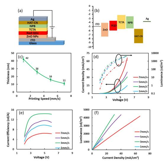
Fig. 3 (a) Schematic device architecture and (b) energy level alignment of PM bottom-emission QLED devices, (c) the thickness of the QD layer in the pixel at different printing speeds, (d) J-V-L characteristics, (e) current efficiency-voltage curves and (f) luminance-current density curves of QLEDs with various printing speeds.
