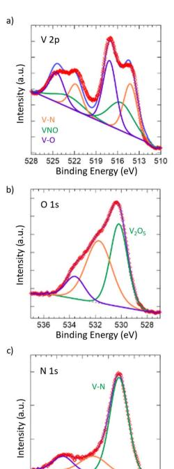
Fig. 2 XPS spectra of (a) V 2p, (b) O 1s, and (c) N 1s for the synthesized VN. All spectra were plotted with respect to reference values. The degree of surface oxidation and amount of pristine vanadium nitride structure were tracked according to the V 2p, O 1s, and N 1s spectra.
