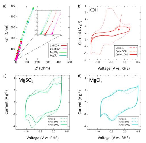
Fig. 6 (a) EIS spectra for 1 M KOH (red), 0.1 M KOH (pink), 1 M MgSO<sub>4</sub> (green) and 1 M MgCl<sub>2</sub> (cyan) with a frequency range of 200 kHz to 10 mHz and an amplitude of 10 mV; (b) stability CVs of VN in (b) 1 M KOH, (c) MgSO<sub>4</sub> and (d) MgCl<sub>2</sub> at 50 mV s<sup>-1</sup> at cycle 1, cycle 500, and cycle 1000.
