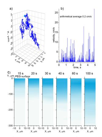
Fig. 3 CFD simulation of the Brownian motion of Cu NPs in PEG: (a) the trajectory of a single Cu NP travelling for 5 s, starting at the position (0,0,0); (b) its instantaneous velocity; (c) 2D Kernel density maps of the collective diffusion of Cu NPs in PEG; the color intensity is proportional to the concentration of the NPs, the NPs are generated randomly within the interval  $-10~\mu m < X < 10~\mu m; Y = 0~\mu m$  at a flux corresponding to the experimentally obtained values.
