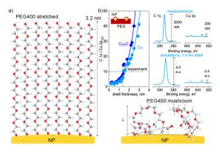
Fig. 13 (a) Two types of PEG400 configuration on the NP surface: high-density brush and low-density mushroom arrangements; (b) SESSA simulations of XPS C 1s and Cu 2p spectra with different thicknesses of the PEG shell over Cu or Cu<sub>2</sub>O NPs; the simulations are compared with the XPS spectra measured on the Cu/PEG nanofluid using an enviro-ESCA.26
