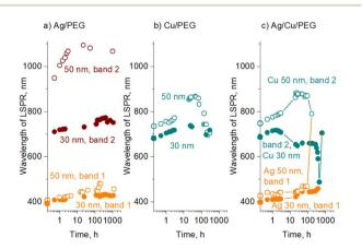
Fig. 7 Change in the LSPR position with time for nanofluids with NPs of mean sizes of 30 and 50 nm: (a) Ag/PEG, (b) Cu/PEG, and (c) Ag/Cu/ PEG. The total metal concentration is 50  $\mu$ g mL<sup>-1</sup> (25  $\mu$ g mL<sup>-1</sup> Ag and  $25~\mu g~mL^{-1}\,\mbox{Cu},$  in the case of Ag/Cu/PEG). Data points placed on the y-axes belong to time = 0 h.
