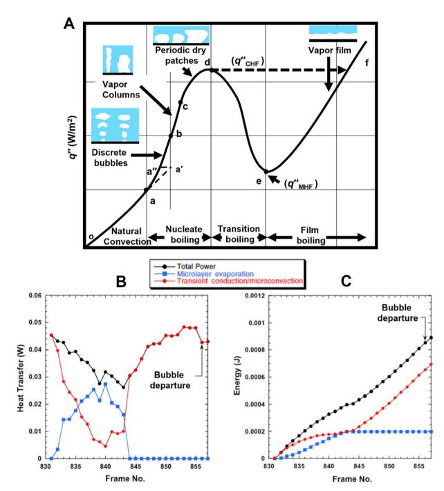
Fig. 1 (A) Heat flux as a function of wall superheat for saturated pool boiling.<sup>28</sup> Relative contributions of microlayer evaporation and transient conduction and microconvection to (B) local heat transfer rate and (C) total energy during nucleate pool boiling under a single bubble.<sup>30</sup> Reproduced with permission from ref. 30. Copyright 2005 Elsevier.
