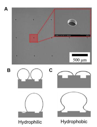
**Fig. 3** (A) SEM images of micro-hole patterned surface.<sup>67</sup> Bubble nucleation and growth on microhole patterned (B) hydrophilic<sup>67</sup> and (C) hydrophobic surfaces at low wall superheats.<sup>67</sup> Reproduced with permission from ref. 67. Copyright 2020 Elsevier.
