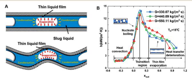
Fig. 9 (A) Top views of confined bubbles in wavy and straight microchannels.<sup>179</sup> (B) Variation of flow boiling HTC (h) as a function of outlet vapor quality ( $x_{out}$ ) for different mass fluxes (G) at an inlet saturation temperature ( $T_{in}$ ) of 15 °C.<sup>179</sup> Reproduced with permission from ref. 179. Copyright 2021 Elsevier.
