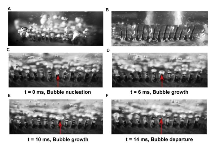
Fig. 4 Optical photograph demonstrating more nucleation for (A) porous structured reentrant cavity surface<sup>88</sup> when compared against (B) nonporous reentrant cavity surface with water as the working fluid.88 (C-F) Bubble nucleation, growth and departure captured for porous reentrant cavity surface with ethanol as the working fluid.88 Reproduced with permission from ref. 88. Copyright 2016 Elsevier.
