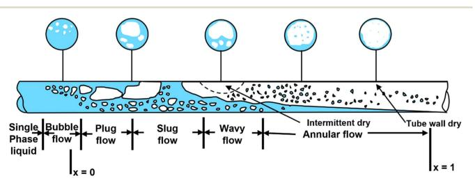
Fig. 7 Subcooled-inlet flow boiling patterns as a function of vapor quality (x) showing bubbly, plug, slug, wavy and annular flow followed by dryout.120
