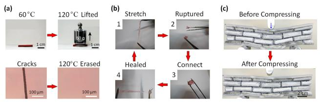
Fig. 8 Self-healing behaviours with (a) a nacre-like architecture based on a dynamic polymer network, (b) the UPy-units doped OEGMA copolymers, and (c) nacre-inspired cement-like materials. Image (a) is adapted from ref. 49. Images (b) and (c) are reproduced from ref. 101 and 24 with permissions respectively from WILEY-VCH Verlag GmbH & Co. KGaA, Weinheim, copyright 2015 and from Elsevier Ltd, copyright 2021.
