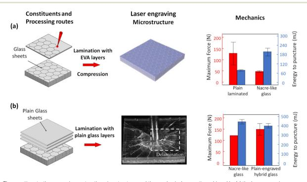
Fig. 6 The constituents, the processing routes, the microstructure, and the mechanical properties achieved by (a) the laser-engraving process. and (b) the combination of laser-engraved and plain glass sheets. The images are reproduced from ref. 4, 10 and 92 with permissions respectively from Springer Nature, copyright 2014, the American Association for the Advancement of Science, copyright 2019, and IOP Publishing Ltd, copyright 2021.
