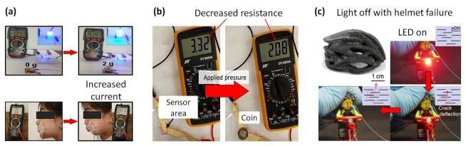
Fig. 9 Force sensing achieved with (a) a nacre-like scaffold made of graphene oxide, MXene, and silk fibroin, (b) a nacre-like material made of graphite and PDMS, and (c) a nacre-like smart helmet made of graphene nanosheets. Image (a) is adapted with permission from ref. 25. Copyright 2021 American Chemical Society. The images (b) and (c) are adapted from ref. 43 and 38.
