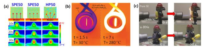
Fig. 12 Heat conductivity and resistance achieved with (a) nacre-like composite made of boron nitride platelets and UHMWPE, (b) nacre-like architectures made of Fe-coated alumina platelets, and (c) 3D nacre-like material made of boron nitride platelets. Image (a) is adapted with permission from ref. 27. Copyright 2018 American Chemical Society. Images (b) and (c) are adapted from ref. 42 and 71 respectively.
