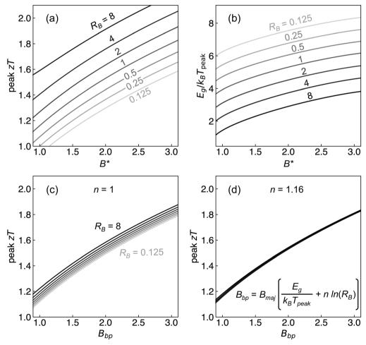
Fig. 6 (a) Peak zT and (b)  $E_q/k_BT_{peak}$  plotted against  $B^*$  (eqn (17)) for different values of  $R_B$ . Peak zT plotted against  $B_{bp}$  (eqn (18)) is shown for (c) n=1 and (d) n = 1.16
