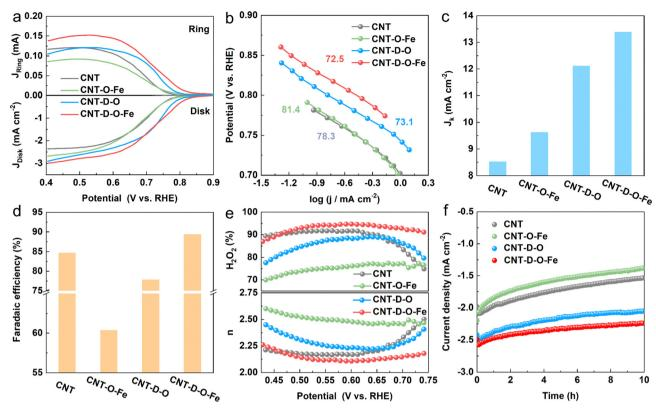
Fig. 4 (a) LSV curves (ring current and disk current density, respectively), (b) the Tafel plots of CNT, CNT-O-Fe, CNT-D-O, and CNT-D-O-Fe; (c)  $J_k$  and (d) faradaic efficiency for  $H_2O_2$  at 0.550 V vs. RHE, (e) electron transfer number and selectivity for  $H_2O_2$ ; (f) stability test of the catalytic materials at 0.550 V vs. RHE.
