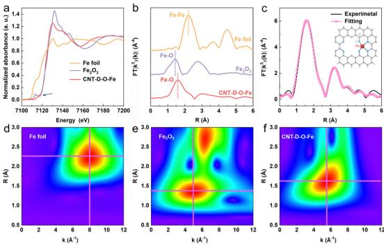
Fig. 3 (a) XANES and (b) FT-EXAFS of Fe foil, Fe<sub>2</sub>O<sub>3</sub>, and CNT-D-O-Fe, the intensity of Fe foil is halved. (c) The fitting curves of Fe K-edge EXAFS spectra of the CNT-D-O-Fe in R space and the optimized Fe-O<sub>4</sub> structure with defects (the inset, gray ball: C atom, blue ball: O atom, red ball: Fe atom). WT plots of (d) Fe foil, (e) Fe<sub>2</sub>O<sub>3</sub>, and (f) CNT-D-O-Fe based on the EXAFS.
