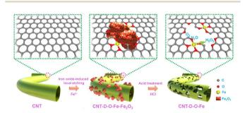
Fig. 1 Schematic of the preparation process of CNT-D-O-Fe.
