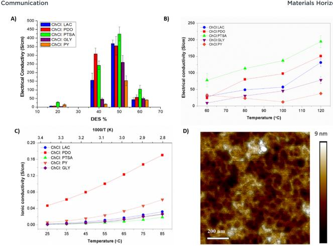
Fig. 2 (A) Electrical conductivities of PEDOT: PSS/DES composites with different DES amounts 20, 40, 50, and 60 wt%, (B) Electrical conductivities of 50/ 50 wt% PEDOT:PSS/DES composites measured by 4PP on dried films, (C) Ionic conductivities of 50:50 wt% PEDOT:PSS/DES calculated throughout fitting at different temperatures and (D) AFM height images of PEDOT:PSS/ChCl:LAC composite films annealed at 120 °C.
