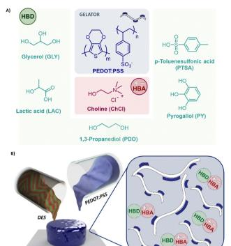
Fig. 1 (A) Chemical structures of PEDOT:PSS and DES used. (B) General pathway for preparing PEDOT:PSS/DES supramolecular eutectogels (left) and scheme of the interactions between the DES (HBA:HBD) and PEDOT:PSS when are mixed between 30 and 60 wt% (right).
