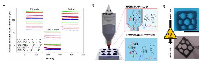
Fig. 3 (A) Dynamic strain tests alternating 1% and 1000% strain at short times of 500 s. (B) Scheme of the DIW method and changes in the interaction of the eutectogel strain function. (C) 3D printed hexagonal patterned PEDOT:PSS/ChCl:LAC eutectogel before and after the annealing process at 50 °C (scale bar = 1 cm).
