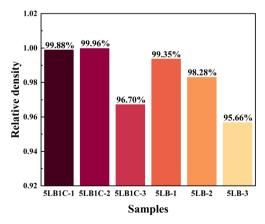
Fig. 8 Relative density of sintered pellets.
