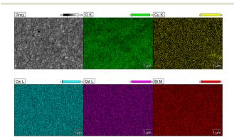
Fig. 7 EDX elemental mapping of the cross-section for the 5LB1C-1
