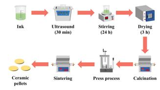
Fig. 1 Fabrication process of the doped GDC pellets.
