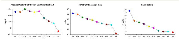
Fig. 4 Comparison of trends in polarity proxies and liver uptakes. Plots were derived from data presented in Fig. 2. Connecting lines between data points are intended only to visualize trends and do not indicate a functional correlation.
