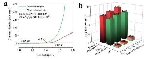
Fig. 6 (a) LSV curves and (b) cell potentials for the electrolysis of water and urea electrolysis with  $\Delta U$  representing the difference in the cell potentials for Cu-Ni<sub>3</sub>S<sub>2</sub>@NiFe LDHs, reprinted with permission from Elsevier, Ding et al. 165
