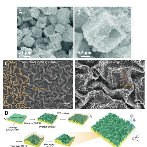
Fig. 5 Approaches employed to minimise the accumulation of gas bubbles at the electrocatalyst surface (A) and (B)  $CoSe_2/MoSe_2$  heterostructures, reprinted with permission from the Royal Society of Chemistry, Chen et al. 118 and (C) wrinkled  $VMoS_2$  and (D) schematic of the wrinkling procedure, reprinted with permission from the American Chemical Society, Jung et al.  $^{122}$
